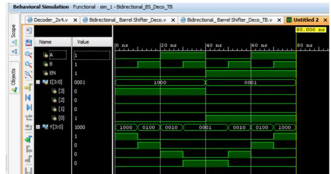
Fig.3(a). Simulation Output Waveforms for proposed Bidirectional barrel shifter
