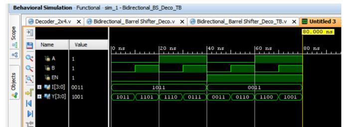
Fig.3(b). Simulation Output Waveforms for proposed Bidirectional barrel shifter.
